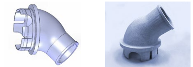
Target interconnector shell after optimisation
