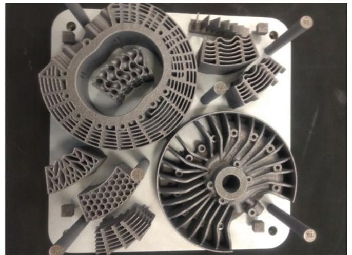
Build bed configuration showing fin geometries
