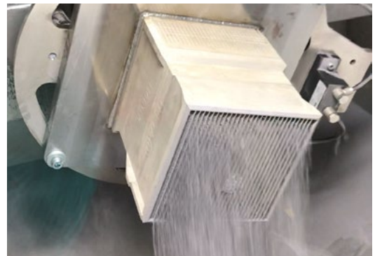
Heat exchanger being loaded & undergoing testing on the Solukon machine
