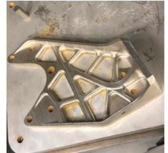
Bracket before separation from build plate
