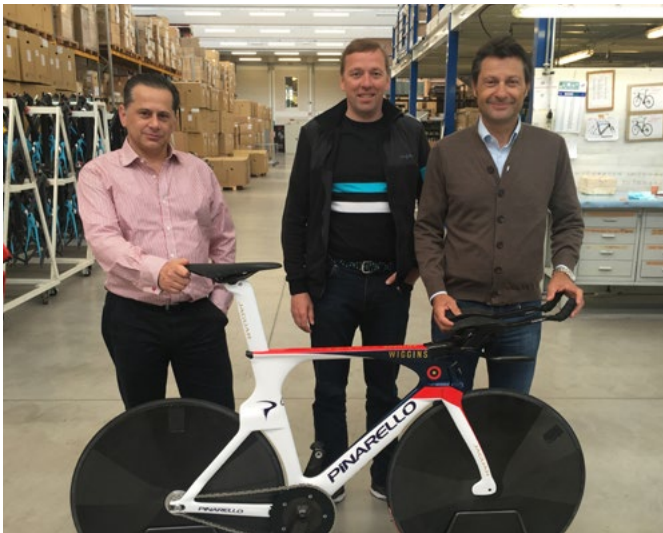
Bradley Wiggins's 2015 Hour Record bike with the revolutionary, first ever, 3D-printed titanium handlebar
